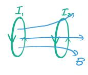
15 consider  $I_1 = I_2 = 0$  initially then gradually increment  $I_1$  is the energy in the B-field is then  $U_1 = \frac{1}{2} L_1 L_1^2$ 4) if Iz is now incremented, it creates  $U_z = \frac{1}{2}L_z I_z$  but also includes an emf in the first oil  $V = \frac{1}{2} L_1 I_1^2 + \frac{1}{2} L_2 I_2^2 + M_{12} I_1 I_2$
