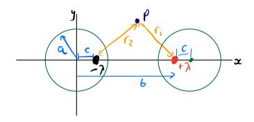
$V(r) = \frac{2}{2\pi\epsilon_0} \ln(\frac{r^2}{r_0}) \Rightarrow \frac{r^2}{r_0^2} = k = const$  for equipotentials. Le expanding out shows that  $c = \frac{a^2}{b}$
