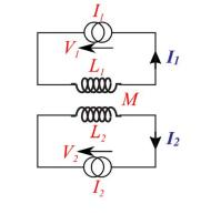
Shence the circuit energy can be derived by circuit analysis. · We can show that L1L2 > M2, or equivalently obtine a coupling coefficient 14=k/LL, 04k=1 4> K=1 means perfect coupling, e.g a doubly wound solenoid.
