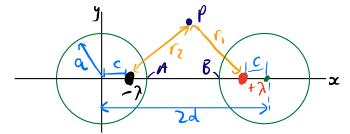
4)  $c = \frac{\alpha^2}{6} = \frac{\alpha^2}{2d-c}$  .  $c = d - \sqrt{d^2 - \alpha^2}$ 4) we can choose easy points A, B to evaluate V Ly the potential is then  $V = \frac{2}{11E_0} \ln \left( \frac{a}{d - \sqrt{d^2 - a^2}} \right)$ Ly in the d>> a limit:  $C = \frac{11E_0}{\ln(2d/a)}$
