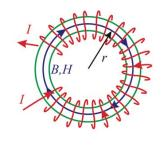
If we introduce an our gap of width L, we can model it as being a different material ( to B field)
