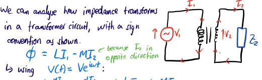
4 then sub Vz = IzZz, eliminate Iz, and newrite in terms of transformer dimensions.
