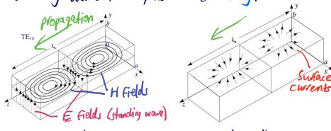
La we can make cuts in the waveguide walls to introduce components, but they must not prevent current flow.
