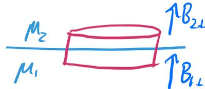
$$\oint_S \underline{B} \cdot d\underline{\zeta} = 0 \Rightarrow B_{1\perp} = B_{2\perp}$$
