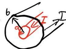
e.g for a pair of narrow wires, we first analyse one wire.  $B(r) = \frac{\mu_0 I}{2\pi r}$
