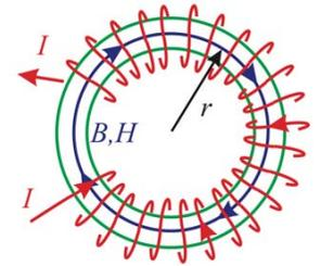
$$\oint \underline{H} \cdot d\underline{l} = \int_S \underline{J} \cdot d\underline{\zeta} \Rightarrow 2\pi r H_{in} = NI \Rightarrow B_{in} = \frac{\mu_r \mu_0 NI}{2\pi r}$$
