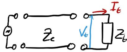
$$V_i = V_1 \exp[j(\omega t - kz)]$$
