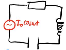
$$V_R(t) = IR = I_0 R \cos \omega t \quad \Rightarrow P = I_0^2 R \cos^2 \omega t$$
