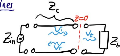
$$Z_{in} = \left. \frac{V_i + V_r}{I_i + I_r} \right|_{z=-a}, \quad I_i = \frac{V_i}{Z_c}, \quad I_r = \frac{V_r}{-Z_c}$$
