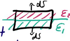
Constructing a loop and using  $\oint \underline{E} \cdot d\underline{l} = 0$ , we must have  $E_{1\parallel} = E_{2\parallel} \therefore D_{\parallel}$  discontinuous.
