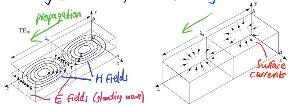
↳ we can make cuts in the waveguide walls to introduce components, but they must not prevent current flow.
