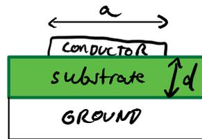
$\hookrightarrow$  hence  $Z$  can be controlled by changing the width of the conductor.
